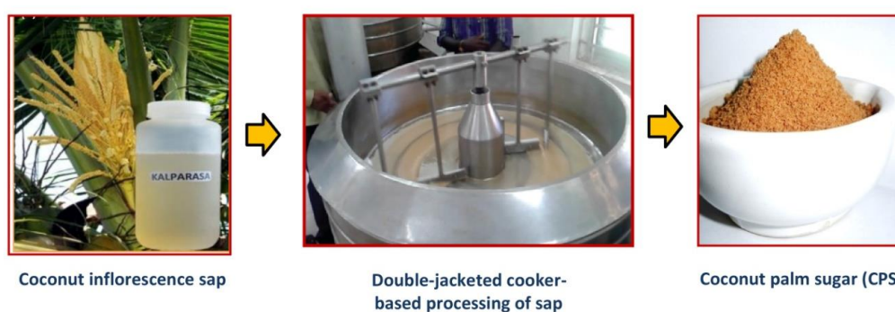
Fig. 1: Process of preparation of coconut palm sugar (CPS) from the freshly collected coconut inflorescence sap ( Kalparasa ® ) using an in-house developed double-jacketed cooker
