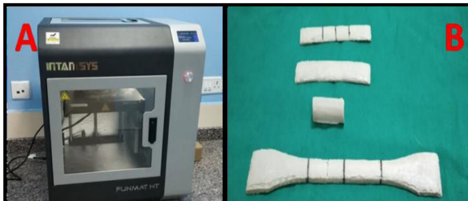
Fig. 1: (A) INTAMSYS - FUNMAT HT 3D printer. (B) 3D printed specimen of PEEK
