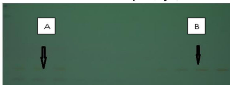
Fig. 2: TLC pigment profile of astaxanthin extracted from Haematococcus cells, (A) Acetone extract. (B) Astaxanthin Standard.
